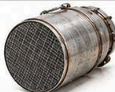
DPF FILTER Traps soot and ash from exhaust gases.
