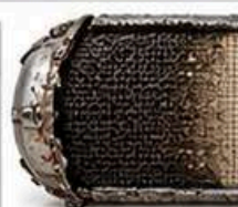
BEFORE CLEANING Soot and ash buildup restricts flow.
